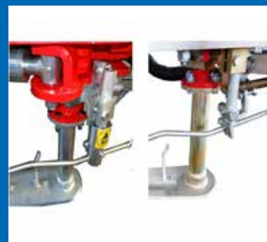
Porta tastatore no-stop / oscillante No-Stop / Oscillating feeler pin holder Porte-tâteur no-stop / oscillant Porta palpador no-stop / oscilante
