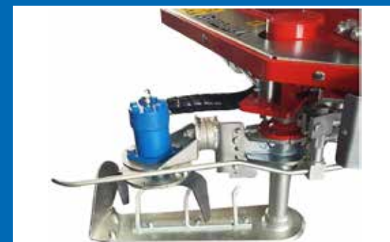
Kit fresino circolare per lama interfilare cm 55 / 65 Circular cutter hydraulic kit for inter-row blade cm 55 / 65 Kit hydraulique fraise circulaire pour lame intercep cm 55 / 65 Kit fresa circular para cuchilla intercepas cm 55 / 65
